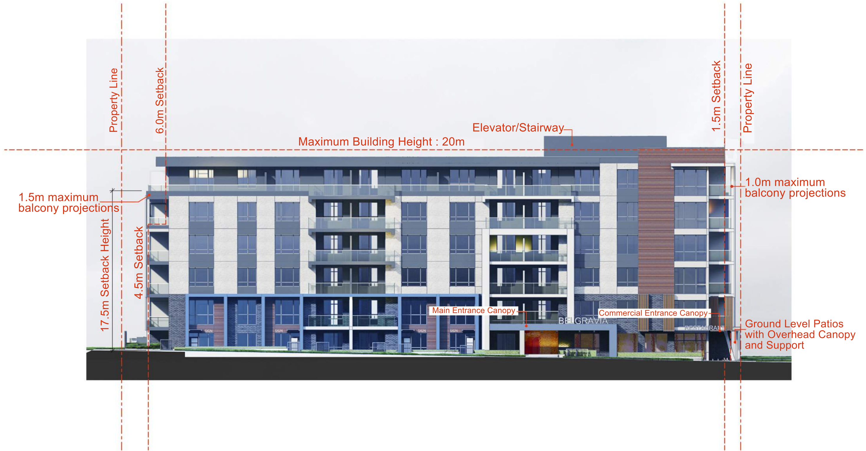
APPENDIX 2a South Elevation
